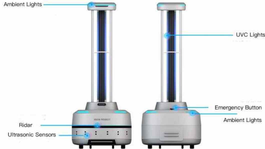
With the detection sensor and emergency stop button, the UVD (UV Disinfection) robot (120-240V/2A Charging Pile Input) is a safe and effective autonomous mobile solution for air and surface disinfection. The product is CE certified for the EU markets. We're doing FCC testing for the US markets it will be soon available.
